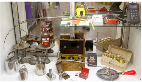
Various tools used by Weights and Measures inspectors to test the accuracy of weighing and measuring devices in the market place.
