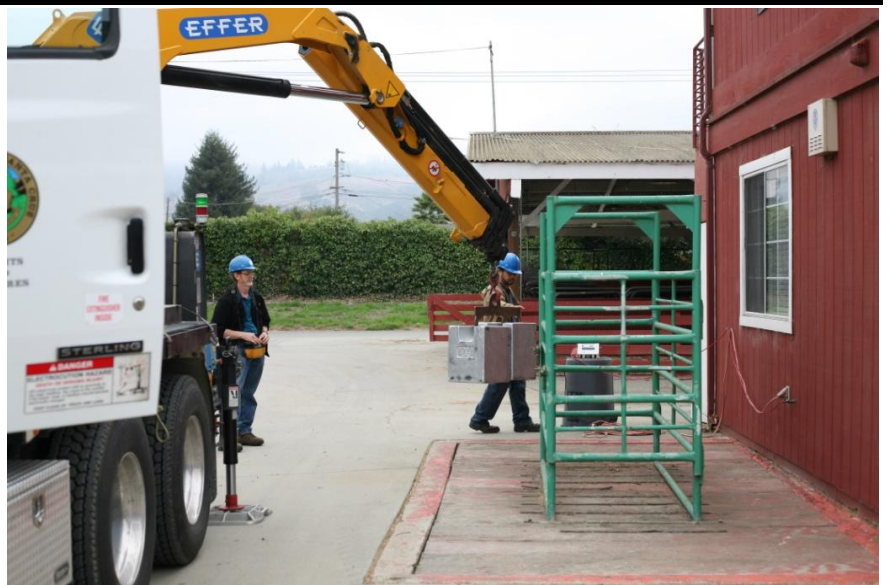
Weights and Measures inspectors testing a livestock scale.
